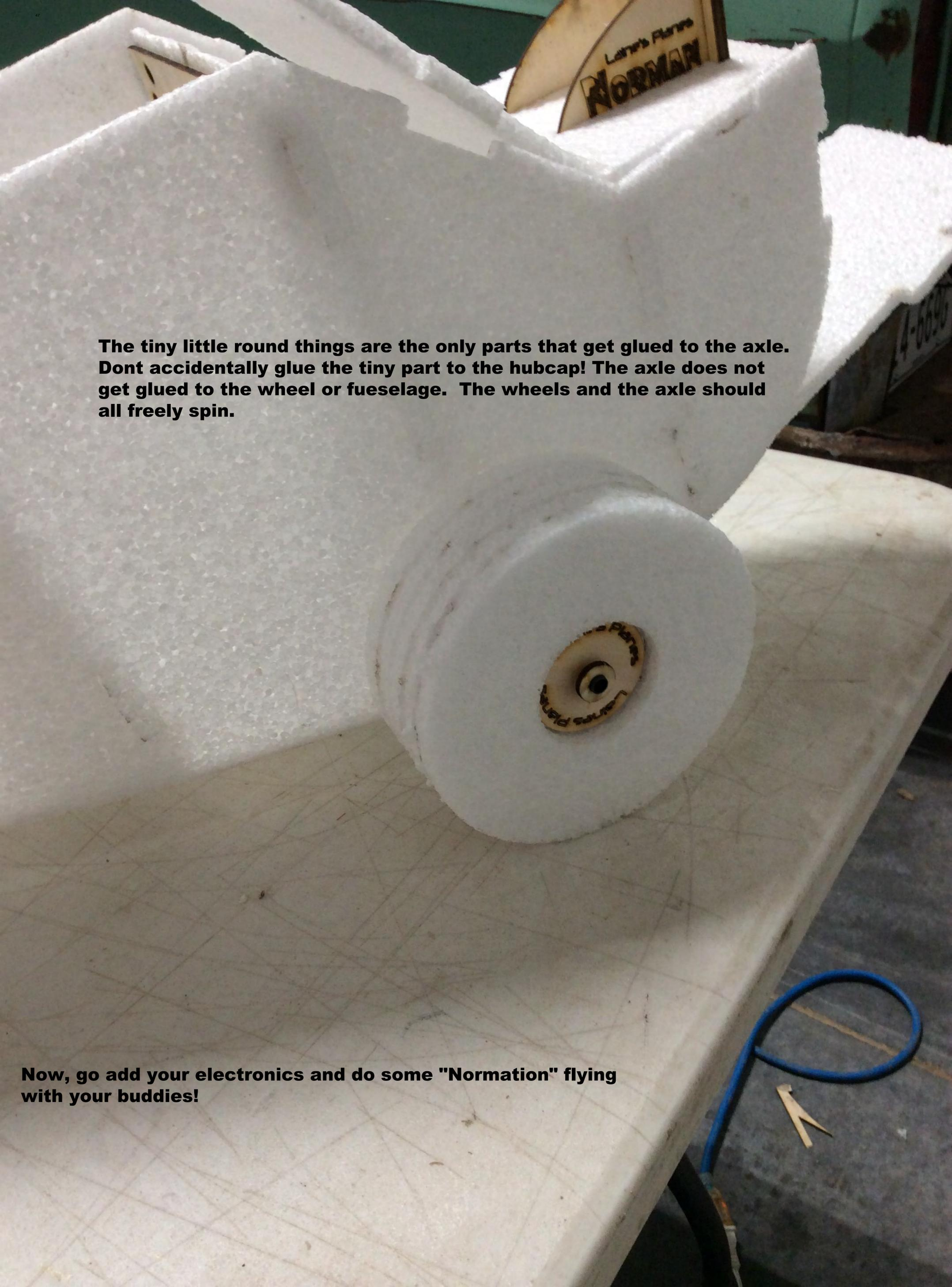
**The tiny little round things are the only parts that get glued to the axle. Dont accidentally glue the tiny part to the hubcap! The axle does not get glued to the wheel or fueselage. The wheels and the axle should all freely spin.**
