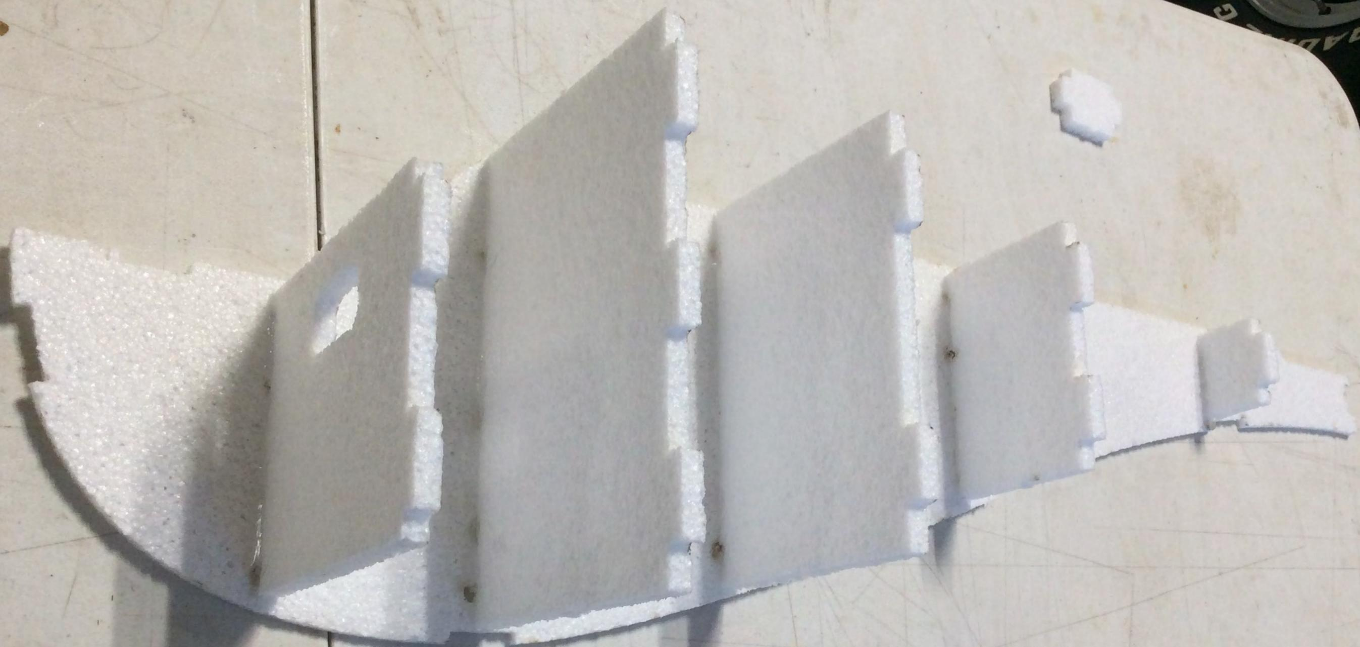
**Get your fuselage bulkheads glued in in this order. I leave the last one out one until the end of the build.**
