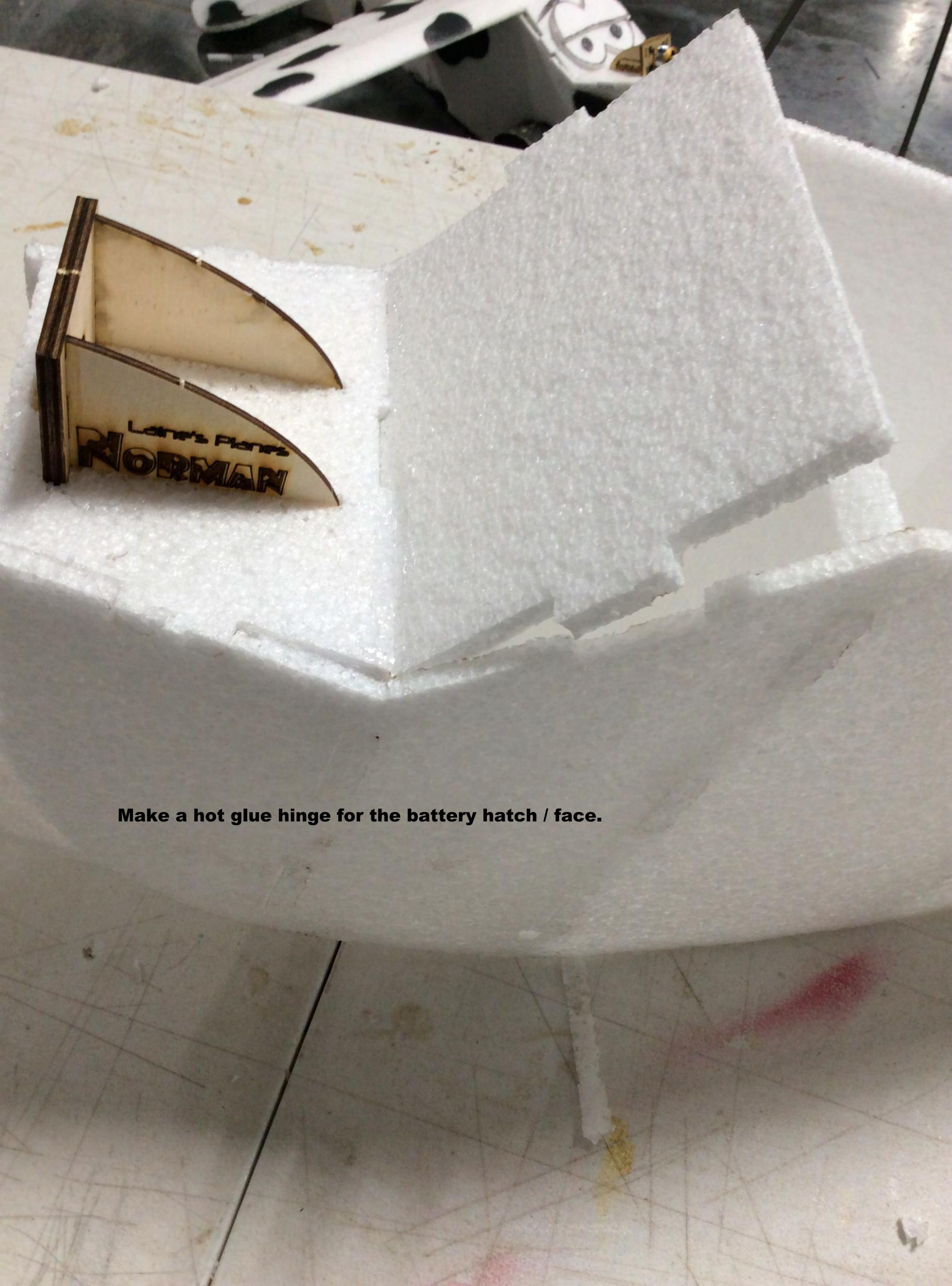
**Make a hot glue hinge for the battery hatch / face.**
