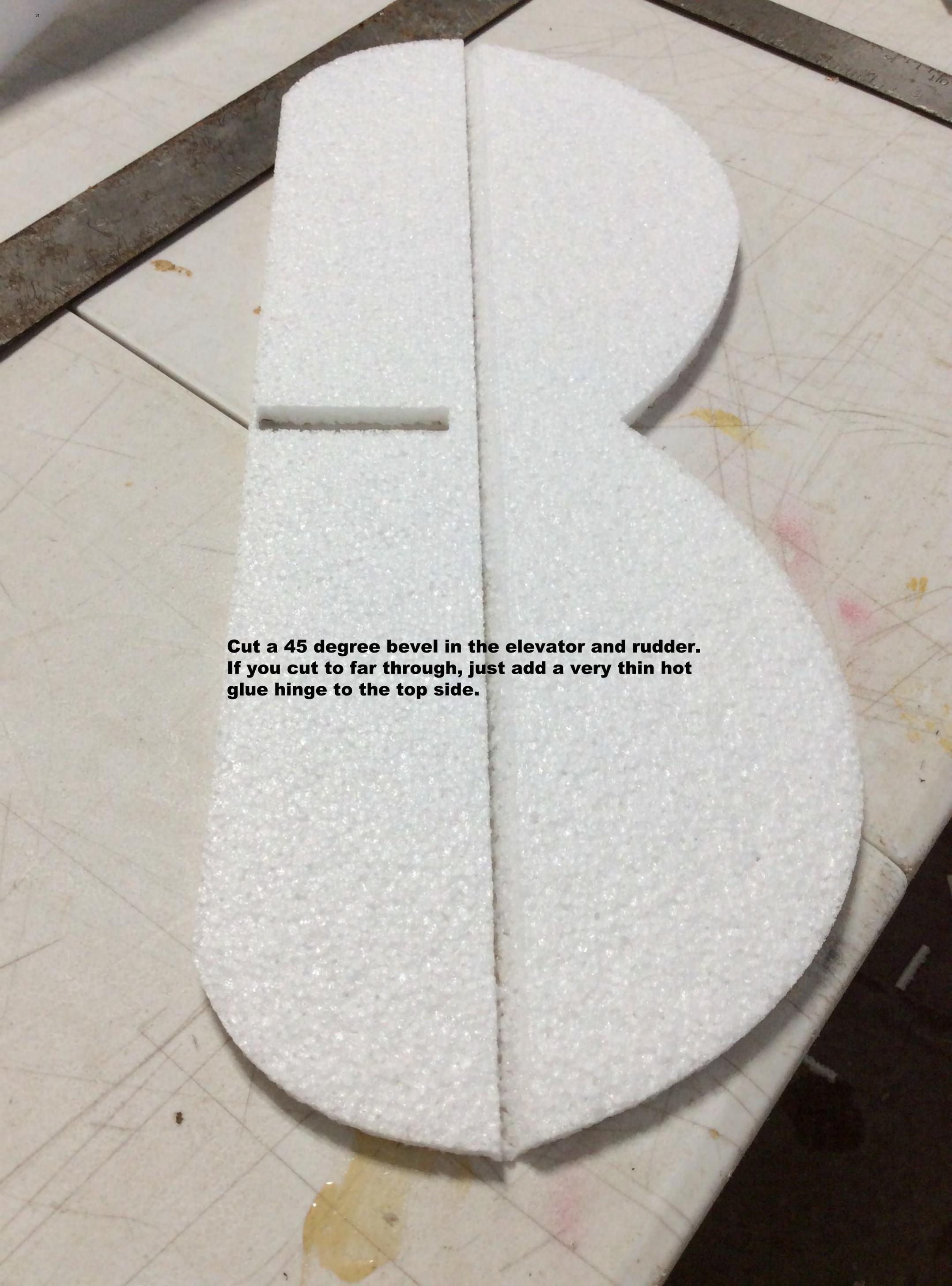
**Cut a 45 degree bevel in the elevator and rudder. If you cut to far through, just add a very thin hot glue hinge to the top side.**
