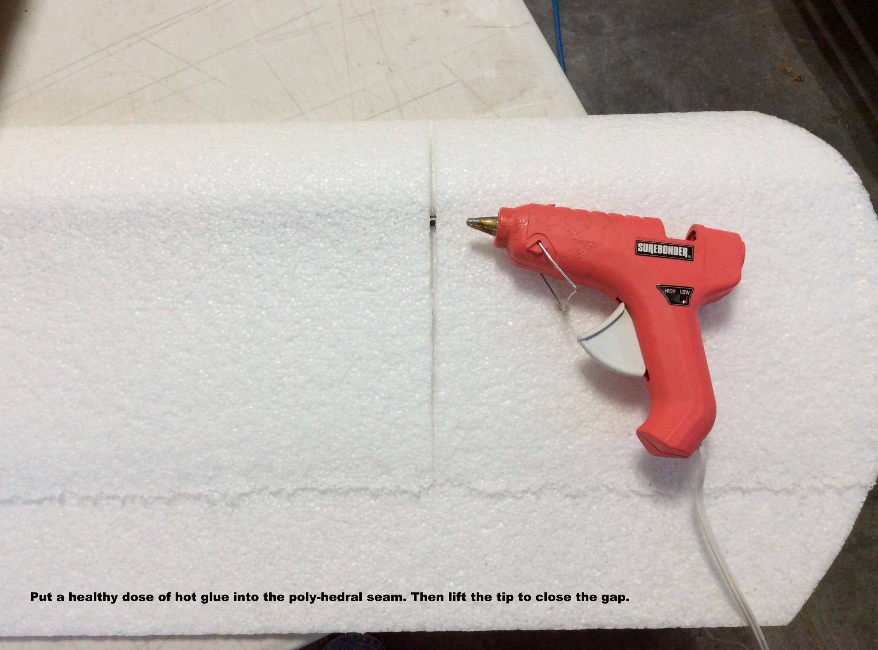
**Put a healthy dose of hot glue into the poly-hedral seam. Then lift the tip to close the gap.**
