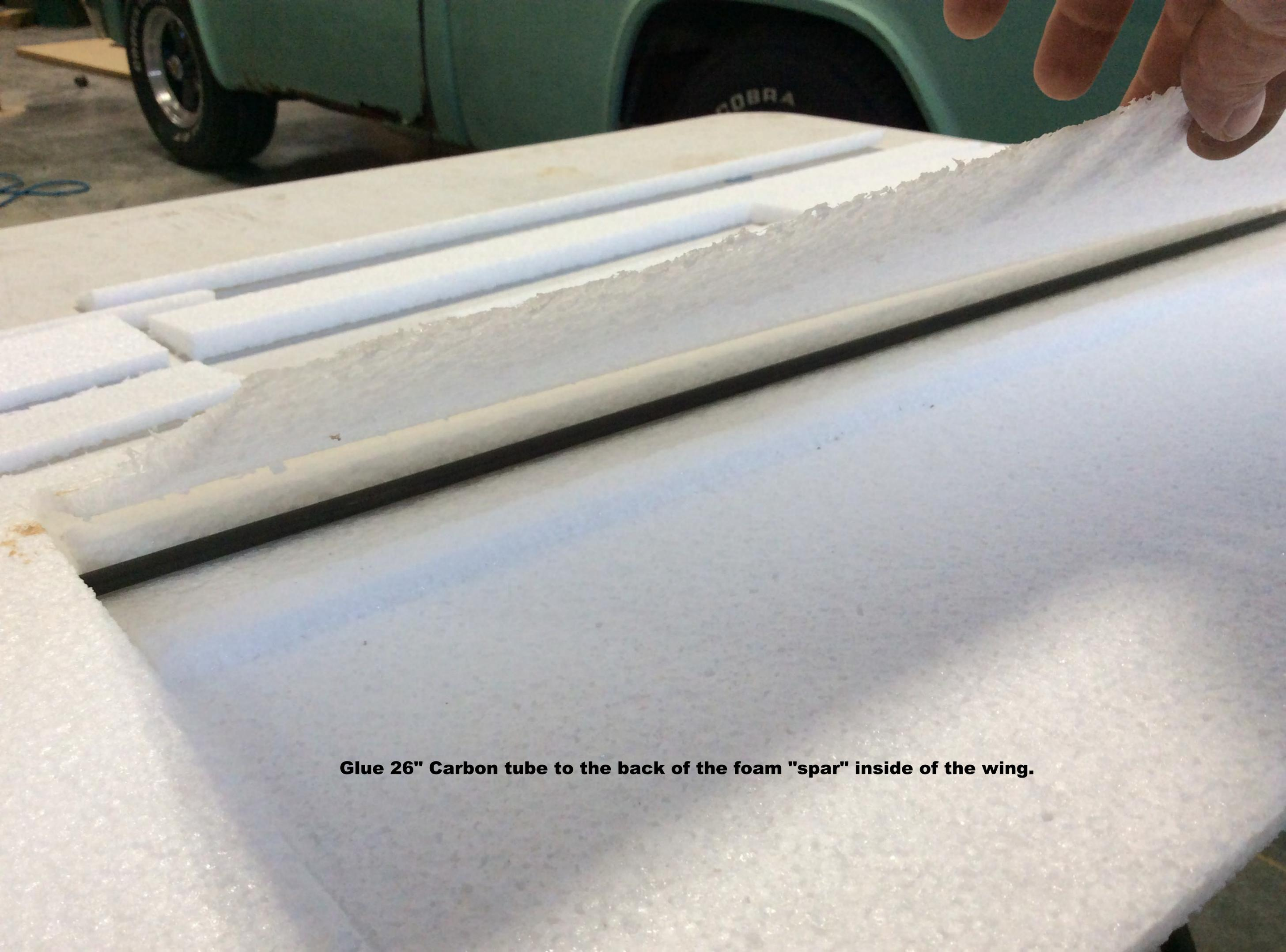
**Glue 26" Carbon tube to the back of the foam "spar" inside of the wing.**
