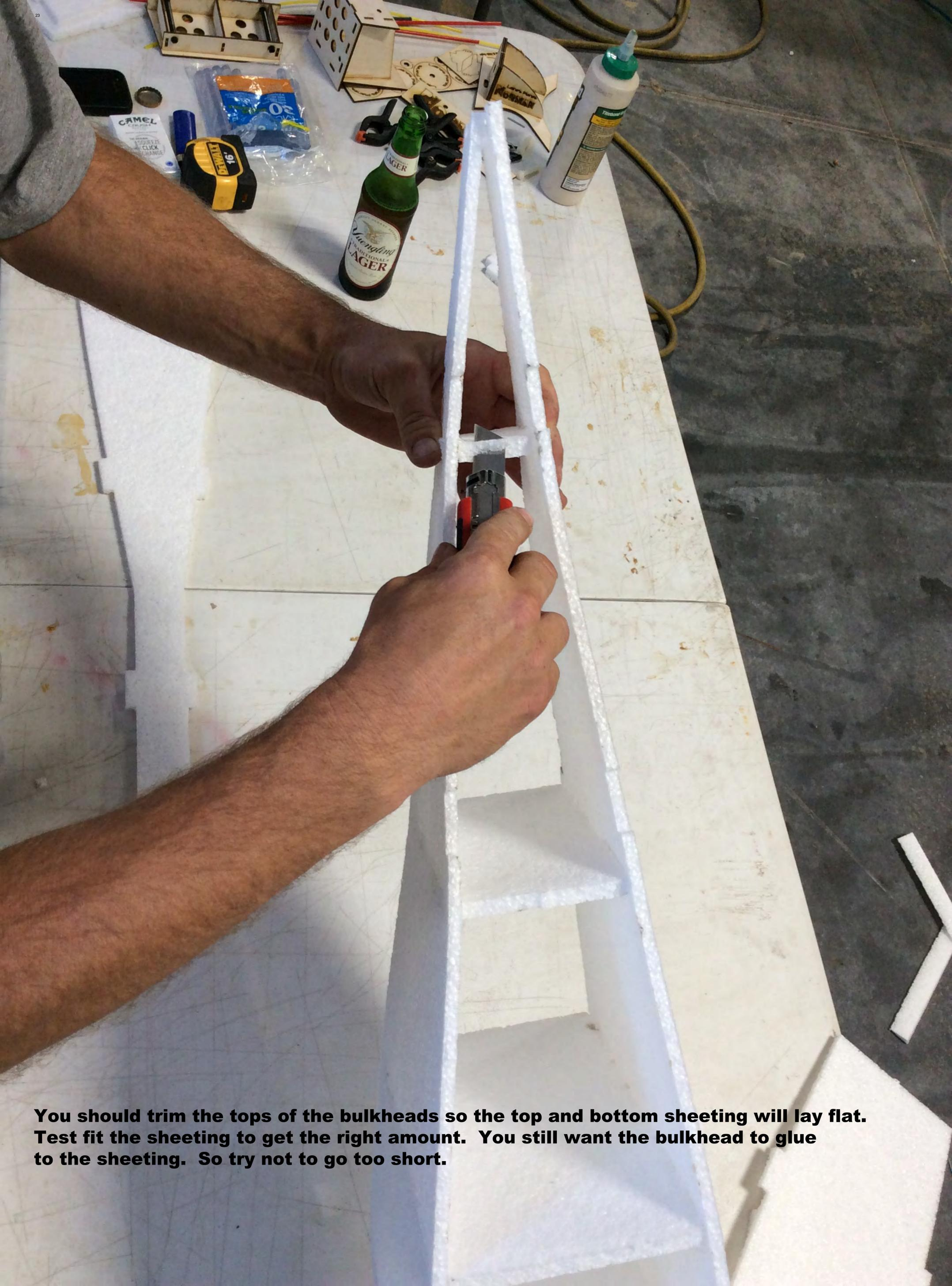
**You should trim the tops of the bulkheads so the top and bottom sheeting will lay flat. Test fit the sheeting to get the right amount. You still want the bulkhead to glue to the sheeting. So try not to go too short.**
